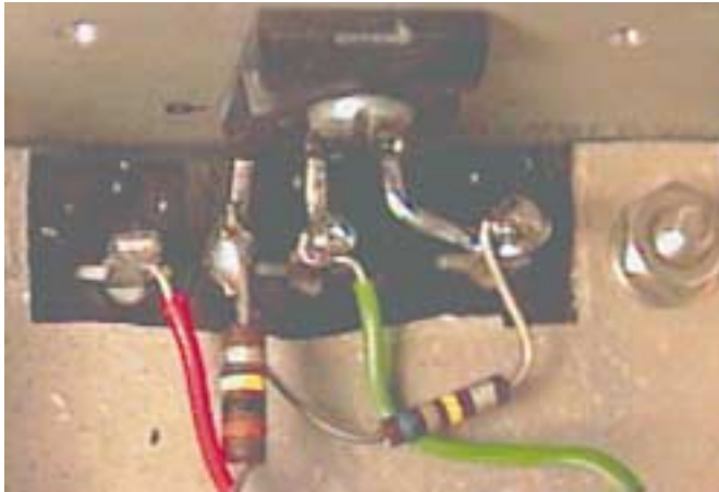
Above: The FET installed.
